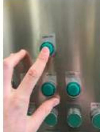
Press the compressor button to supply your air tanks with a additional air supply
