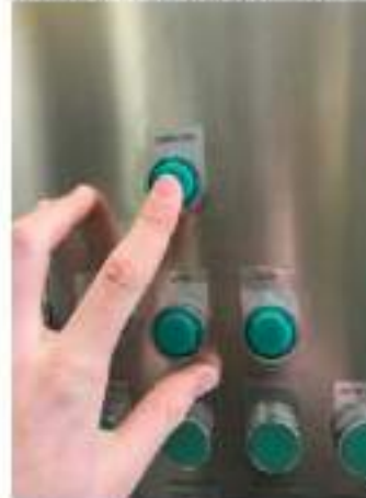
Press the compressor button to supply your air tanks with a additonal air supply
